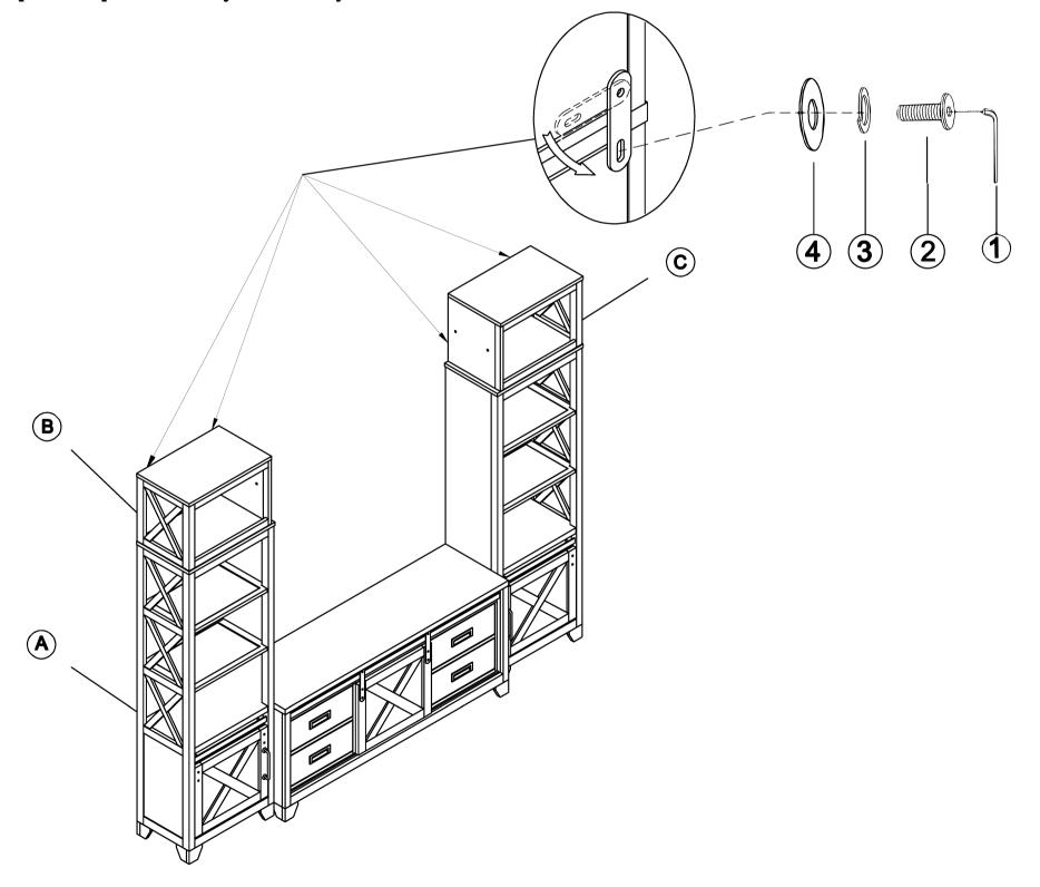
STEP 1: Place the assembled storage bridge Ends(L/R) onto the piers and secure with Connector Plates and Metal hardware as shown.
