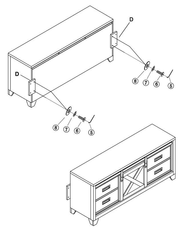
STEP 4: Attach the connect panels(D) to the back of the console using the provided hardware as shown
