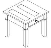
STEP 1: Place the top (A) up side down on the soft surface such as carpet and pull out the drawer.
