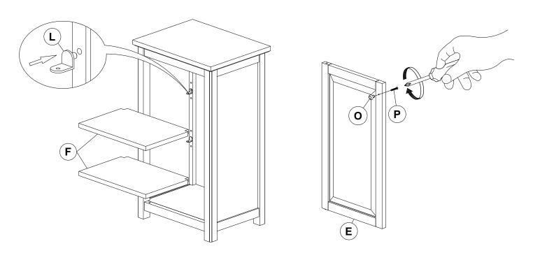
Attach door (E). Insert 40MM Bolt (K) into Threaded Insert in underside of rail on Top Assembly. Align hole on Top of Door (E) with 40MM Bolt (K). Align Washer (J) between Holes on Bottom of Door and upperside Bottom Frame (D). Thread 1-M6x45MM Hex Bolt (I) thru rail on Bottom Frame (D) and Washer (J). Align into Hole on Bottom of Door (E).
