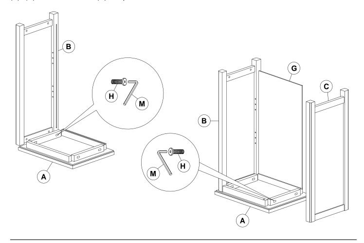
Attach Bottom Frame (D) to Side Frame Assembly (B)&(C) using 4-M6x35MM Hex Bolts (H). NOTE: TIGHTEN ALL BOLTS AT THIS TIME!
