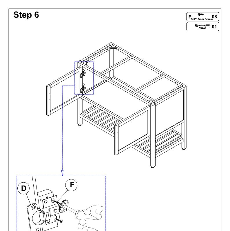
Align slotted holes in Hinge Mounting plate on 2 doors with pilot holes on Side Panel(2) & (3) . Attached 2 Doors using
