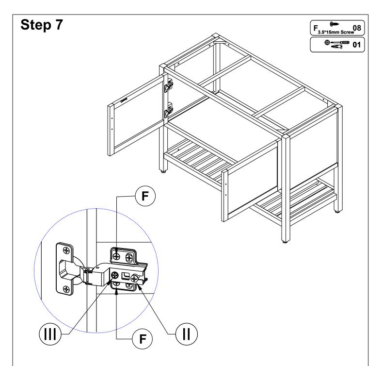
If any hinge requires slight adjustment out, loosen Bolt II and adjust out as necessary.
