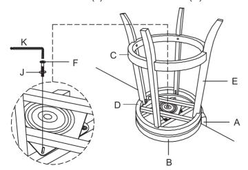
Stand chair up on an even surface and check that it is balanced. If there is a slight wobble, apply downward pressure in the corner where a leg is uneven. Keeping pressure in that corner, tighten all bolts. If balanced, apply downward pressure evenly in the center and tighten all bolts. Do not over-tighten beyond hole depth.
