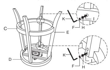
Take the Allen Wrench, and turn the bolts until the legs are secure. DO NOT TIGHTEN COMPLETELY. Stop when you feel you are adding force to tighten the bolt.
