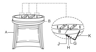
Keep the Backrest (A) and Cushion Seat (B) inverted on a stable raised surface. Attached the Swivel Plate located on the Apron With Swivel Plate (D) to the Cushion Seat (B) using Bolt (F), Flat Washer (J) with Allen Wrench (K). Turn the Swivel Pub Stool right side up.
