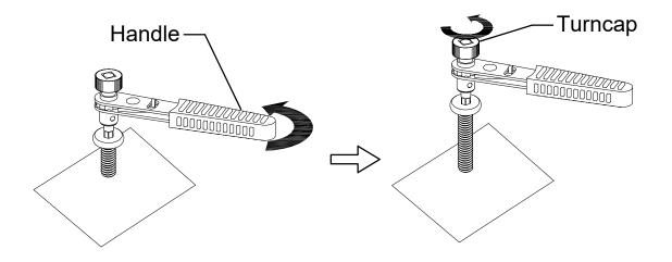
Attach Rail Support Bar (C) to Rail Sections (A) & (B), insert the Bolt (H), turn the Ratchet Tool (J) to tighten them.
