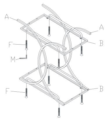
Attach Railing (C) to Metal Frame (B) by Bolt (F) and Allen Wrench (M) as shown.
