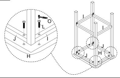
Stand stool up on an even surface and check that it is balanced. If there is a slight wobble, apply downward pressure in the corner where a leg is uneven. Keeping pressure in that corner, tighten all bolts. If balanced, apply downward pressure evenly in the center and tighten all bolts. Do not over-tighten beyond hole depth.
