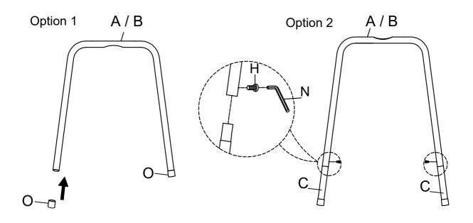
2 Put Upper 'U' Tube (A) into the groove of Lower 'U' Tube (B).
