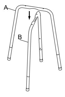
Turn the Swivel (D) 45 degrees (as picture shown) for easy assembly. Then put it on Upper 'U' tube (A) & Lower 'U' tube (B), align the holes and firmly tighten with (I), Lock Washer (L) and Flat Washer (M) using Allen Key (N).
