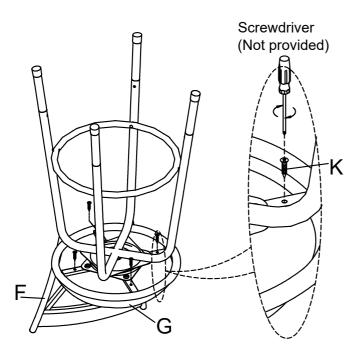
Stand chair up on an even surface and check that it is balanced. If there is a slight wobble, apply downward pressure in the corner where a leg is uneven. Keeping pressure in that corner, tighten all bolts. If balanced, apply downward pressure evenly in the center and tighten all bolts. Do not over-tighten beyond hole depth.
