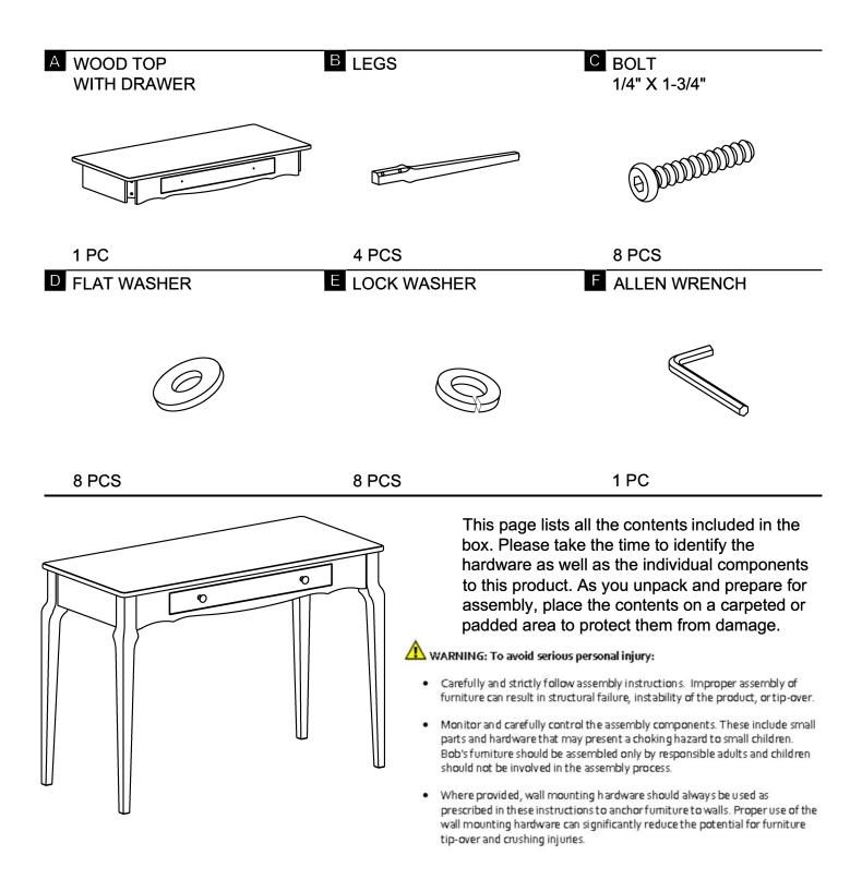
Attach legs (**B**) to wood top (**A**) by using bolt (**C**), lock washer (**E**), flat washer (**D**) and allen wrench (**F**) as shown.
