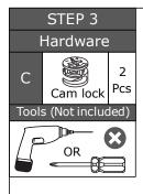
With the pieces placed oriented as shown, ensamble the partition panels 7 and 9 to the shelf 8 with cam locks C as explained in the **TUTORIAL PAGE**.
