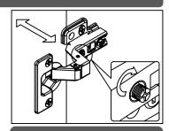
To adjust side-to-side, loosen up or tighten this screw.
