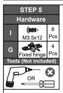
Pay attention to the orientation of the fixed hinges **G**, and attach them to the side panels **6** and **10** with screws **I**.
