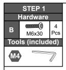
Assemble the first left shelf **12** to the middle bars on the frames **1** and **2** with screws **B** from underneath.
