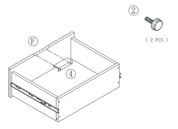
To insert the DRAWER into your unit, line up the EXTENSION SLIDES on the drawer with the EXTENSION RAILS on the unit and push the drawer into the unit until the drawer is fully inserted.
