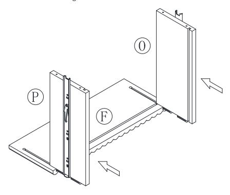
◆ Slide the DRAWER BOTTOM (K) into the grooves, in the DRWAER SIDES (O and P), and the DRAWER FRONT (F).
