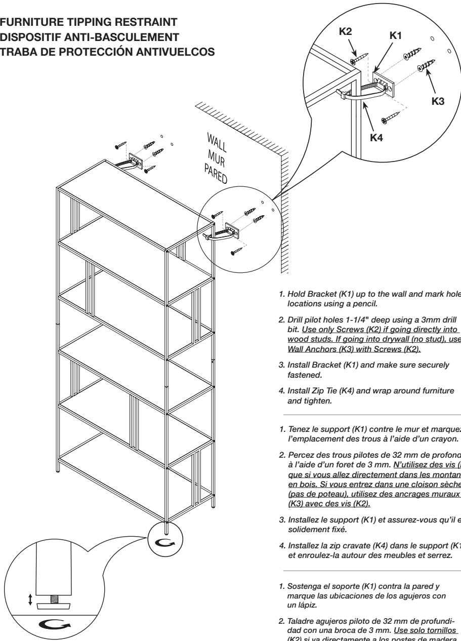
**NOTE:** Use the leveling feet to make sure furniture is level on the floor before using.
