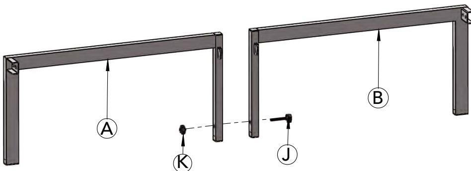
Attach parts (A) and (B) together as shown using bolt (J) and nut (K).
