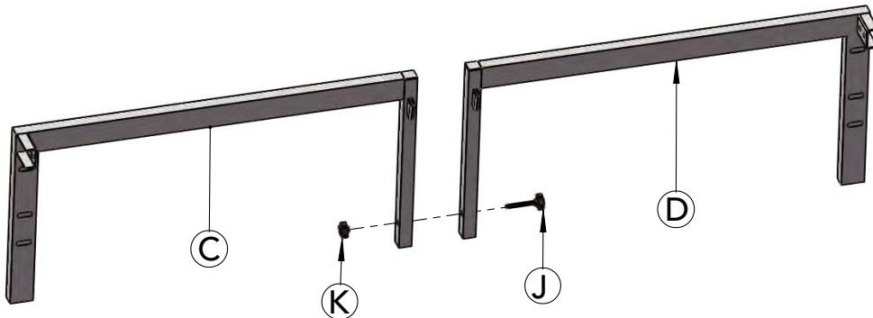
Attach parts (C) and (D) together as shown using bolt (J) and nut (K).
