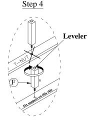
Attach Center Support leg (F) to slats (E) on the side with No Visible T-Nut head
