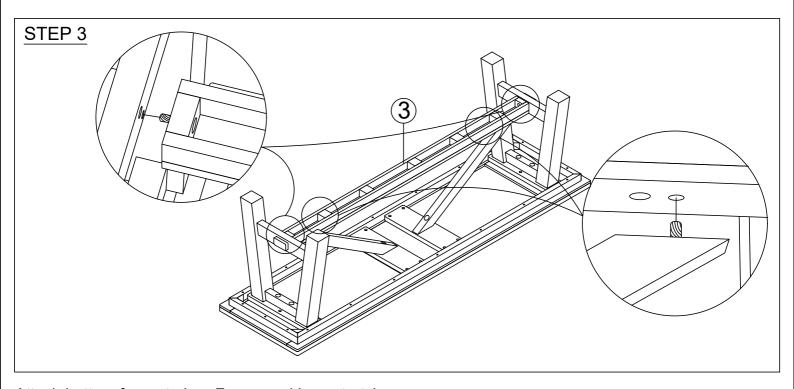
Attach bottom frame to Leg Frame and long stretcher.
