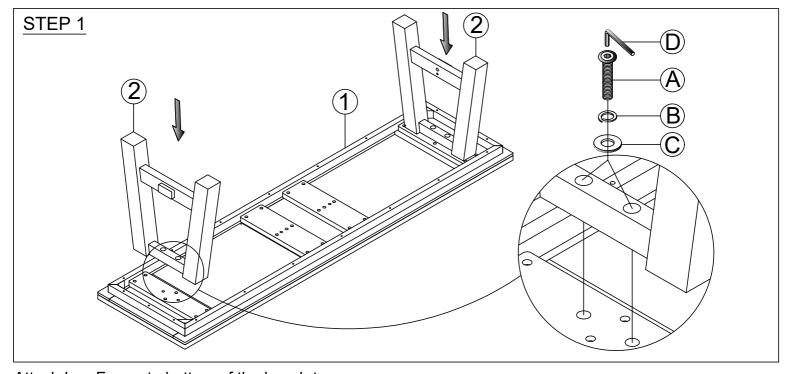
Attach Leg Frame to bottom of the bench top. Note:Do not tighten all bolts until the bench is fully assembly .
